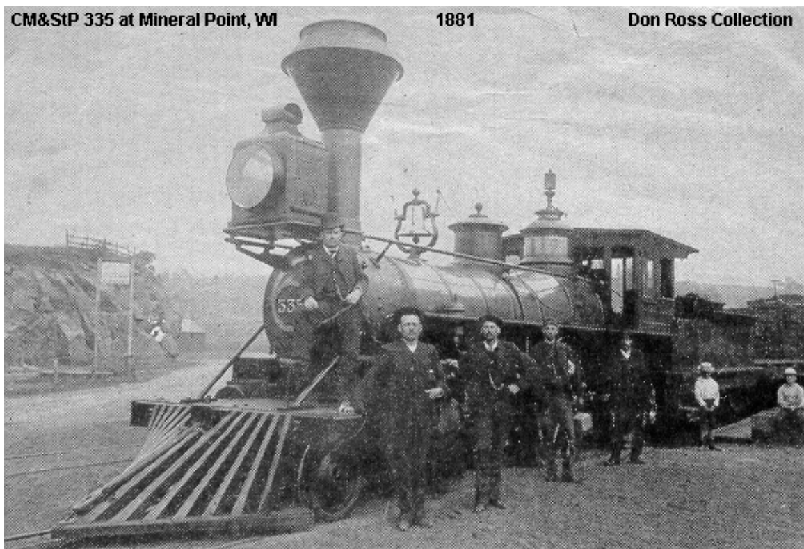
Figure 1: This 4-4-0 locomotive was built for the Chicago & Pacific and then labored for the Chicago, Milwaukee & St. Paul after the 1880 buy-out. Source: Don Ross collection. http://donsdepot.donrossgroup.net/dr385.htm
